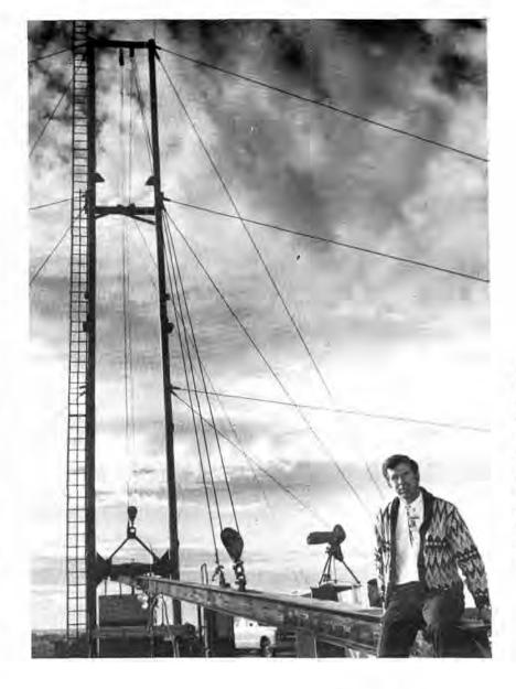
LAUNCHER, ROCKET, Erector Set, is what this arrangement is all about. Marv Timmerman of Tracks and Guns Division 9333 is designer. When end of I-beam Marv is sitting on is elevated, test vehicle suspended under beam is propelled by rockets down into target at whatever angle of impact desired. New facility is located in Area III.
